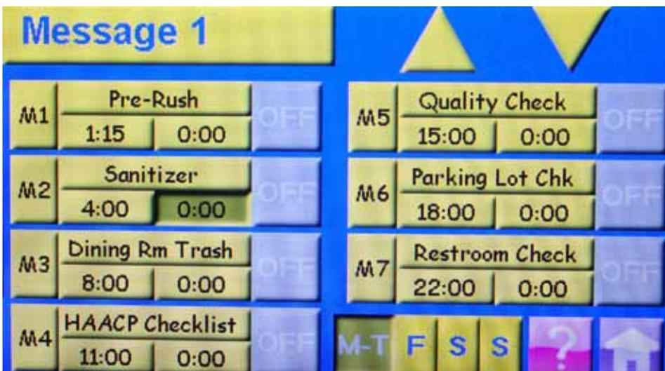
Set repeat interval- the time in minutes when the message will play again in the headset. Select the button next to the start time and then use the arrows to adjust the interval time.
