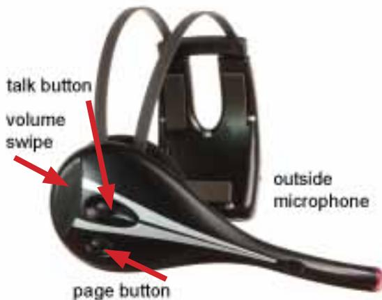
The WT headset features three (3) electronic touch “buttons” that sense the presence of a finger. No pressure is required as there are no moving parts. Only one button at a time may be activated.
