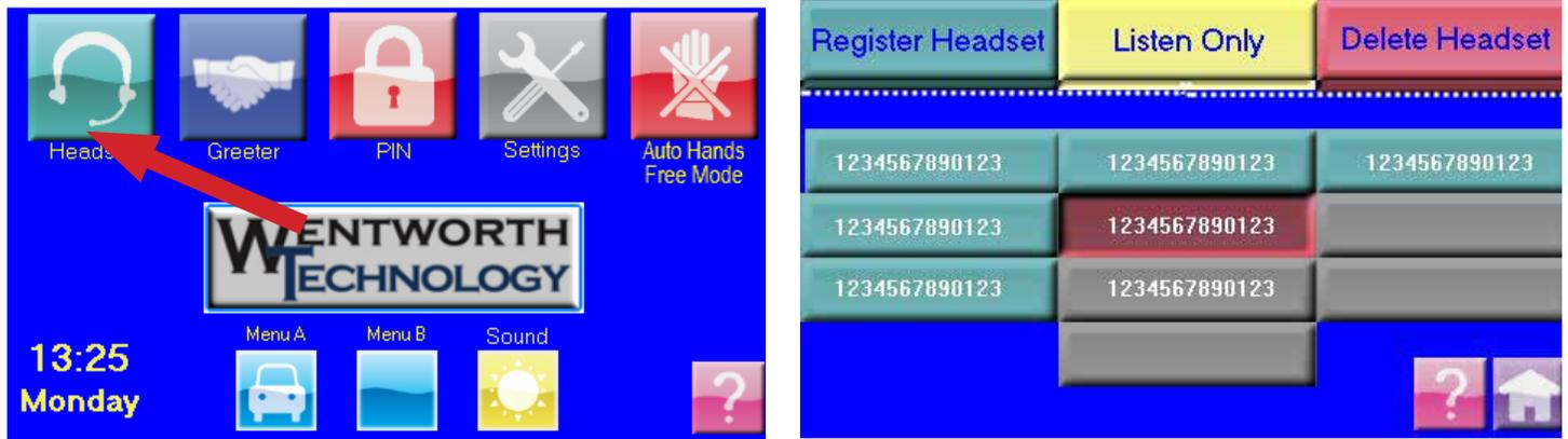
In order to prevent unintended communication between a headset and the order point, use the Listen Only Option, which disables the Center button but allows the Page button to function. When the headset is powered on or if the center button is pressed a voice prompt of “Listen Only Mode” is played to remind the user of limited operation.
