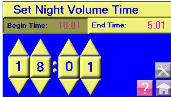
Press "Begin Time" or "End Time" and adjust the time using a 24-hour format. (6:01 PM would be entered as 18:01.)
