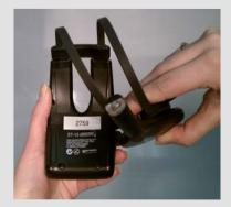
Headset size can be adjusted by sliding the headband in or out of the battery side. To adjust grip of the headset on your head, twist headband in and past the opposite side as shown.
