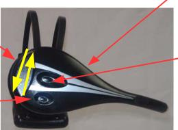
Microphone boom rotates up and over for left or right ear wearing style.
